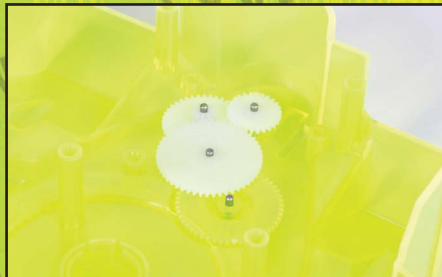
FIGURE 14. Flip the top cabinet over and install the program disk gear drive train.
